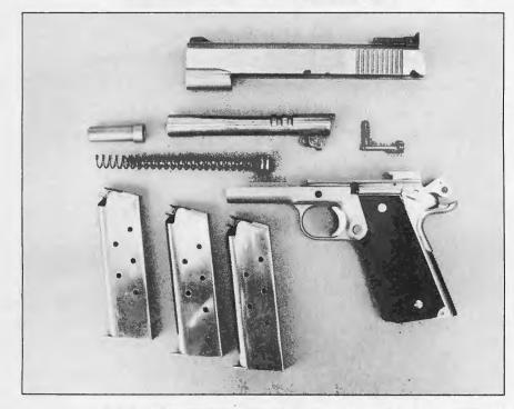
**ABOVE: Clean and** simple, stripped Score Master shows fewer parts, more stainless than ordinary .45. **RIGHT:** Most everything a competitor could want: Commander hammer, ambidextrous safety, extended grip safety, flat mainspring housing and Pachmayr stocks. LOWER **RIGHT: Bull** barrel and guide rod distinguish **Detonics** competition pistol.
